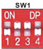
Dip switch module on controller PCB
