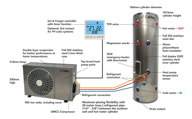
The stainless steel hot water cylinder fits inside your standard hot water cupboard or can be positioned outside. The KP-50 outdoor unit has a heating output of 4 kW with a nominal power use of just over 1 kW. The coefficient of performance (COP) is 4, and we use R32 refrigerant. The heat pump will heat the water up to 60°C.
